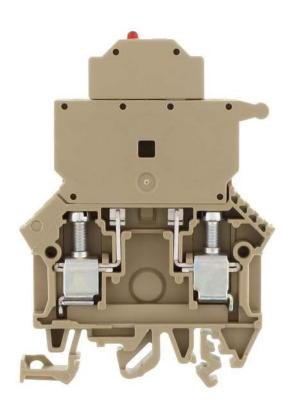
Fuse-disconnect terminal, Screw connection, Mounting type:Mounting rail TS 35/7.5 and TS 32, Rated cross-section: 10 mm², Width: 8 mm, Colour: Beige
