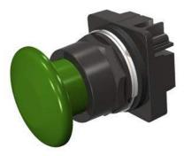
30mm BlackMax, Epoxy Coated Corrosion Resistant Metal Operator, Round Push-Pull Operator Non-Illuminated Mushroom Head Cap Small 1 3/4" (44.5 mm) Plastic, Green 3 Position Pull-Momentary/Push-Maintained UL Listed, CSA Certified NEMA 1,3,3R,4,4X,12,13 & Automotive Standards
