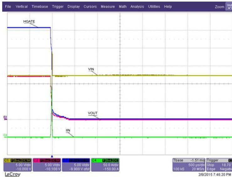
Figure 3. Hot Short With No Load on VOUT (Zoomed Out)
