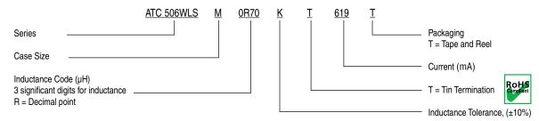
The above part number refers to a 506WLS Series, Case Size M, 0.70 µH inductor, K tolerance (±10%, typ.), with Tin Termination (T), 619 mA, tape and reel packaging...
