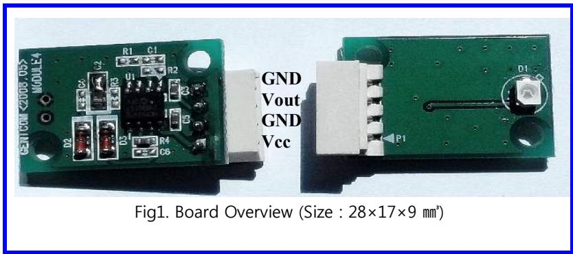
Fig1. Board Overview (Size : 28x17x9 mm<sup>3</sup>)
