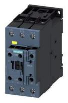
power contactor, AC-3e/AC-3, 51 A, 22 kW / 400 V, 3-pole, 83-150 V AC/DC, 50/60 Hz, with integrated varistor, auxiliary contacts: 1 NC, screw terminal, size: S2, F-PLC-IN
