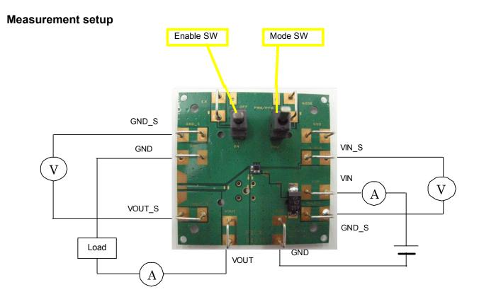
The enable switch has three positions.
