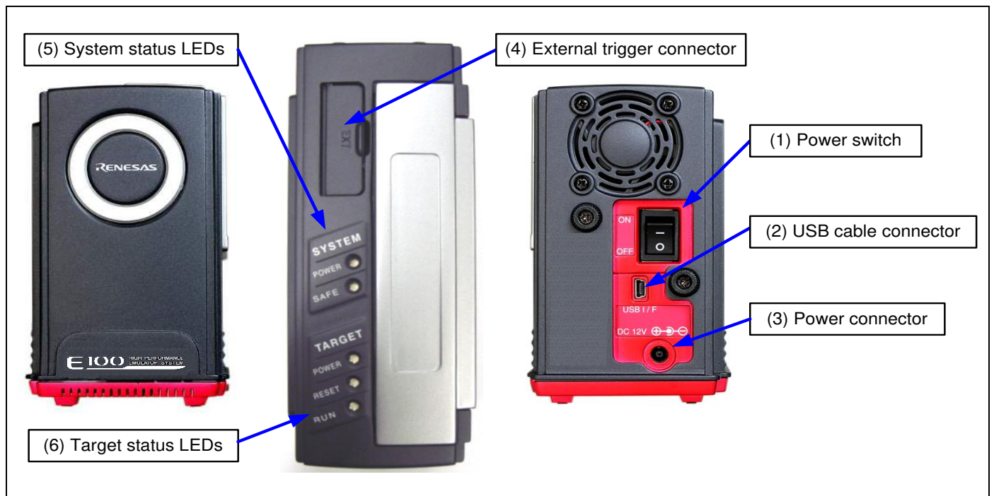
Figure 1.2 Names of each part of the emulator
