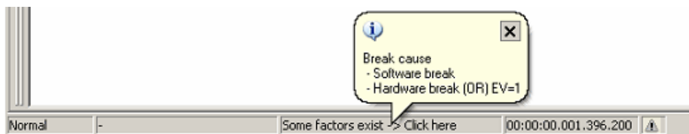
Figure 5.14 Example of break factors display when break factors occur
