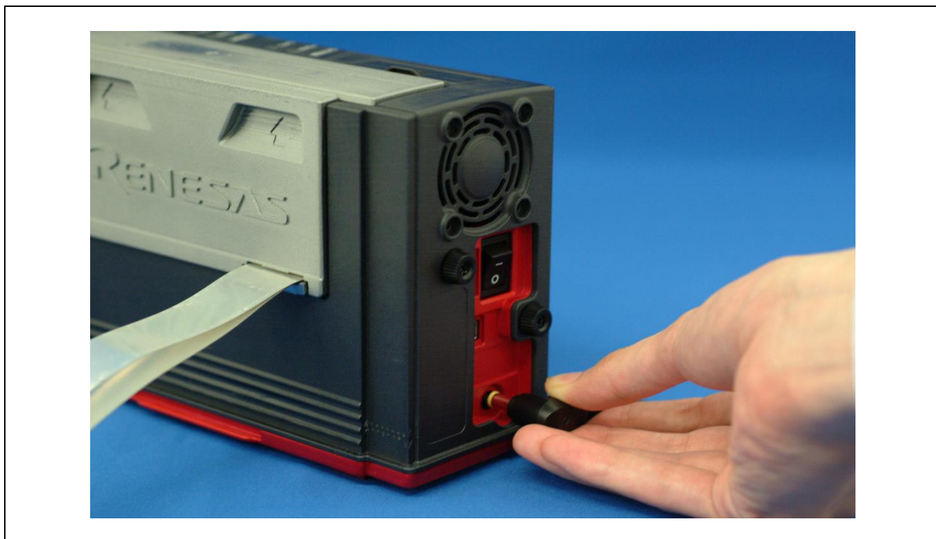
Figure 2.5 Connecting the emulator power supply
