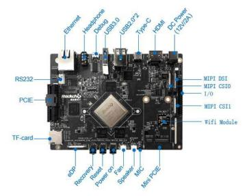
The TB-RK3399Pro development board has rich external interfaces, including 4 lanes PCIE and Mini PCIE, dual high-speed USB3.0 port Type-C + USB3.0 Type-A, dual MIPI CSI and dual ISP with pixel processing capability up to 1300W pixels, and HDMI2.1, DP1.2, MIPI-DSI and EDP; it also supports 8-channel digital microphone array input.
