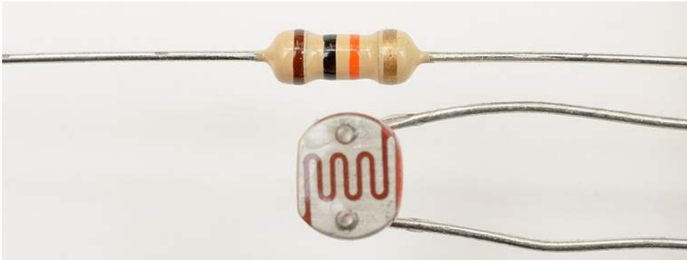
10 kΩ resistor (top), LDR (bottom)
