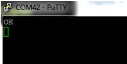
Figure 32: Radio modem sends “OK” prompt through serial link when AT Command Mode is Enabled
