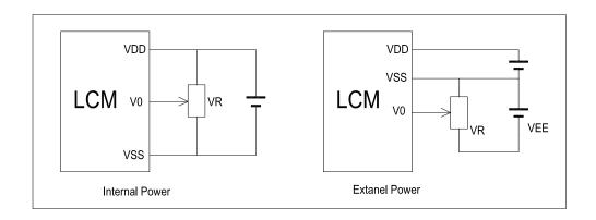
$V_{DD^{\sim}}V_0$ : LCD Driving voltage
