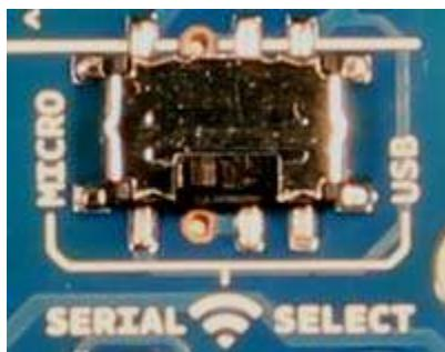
With the switch in the USB position, the DOUT pin the wireless module is connected to the RX pin of the USB-to-serial converter, and DIN on the wireless module is connected to the TX pin of the USB-to-serial converter. This means that the module can communicate directly with the computer. The microcontroller on the
