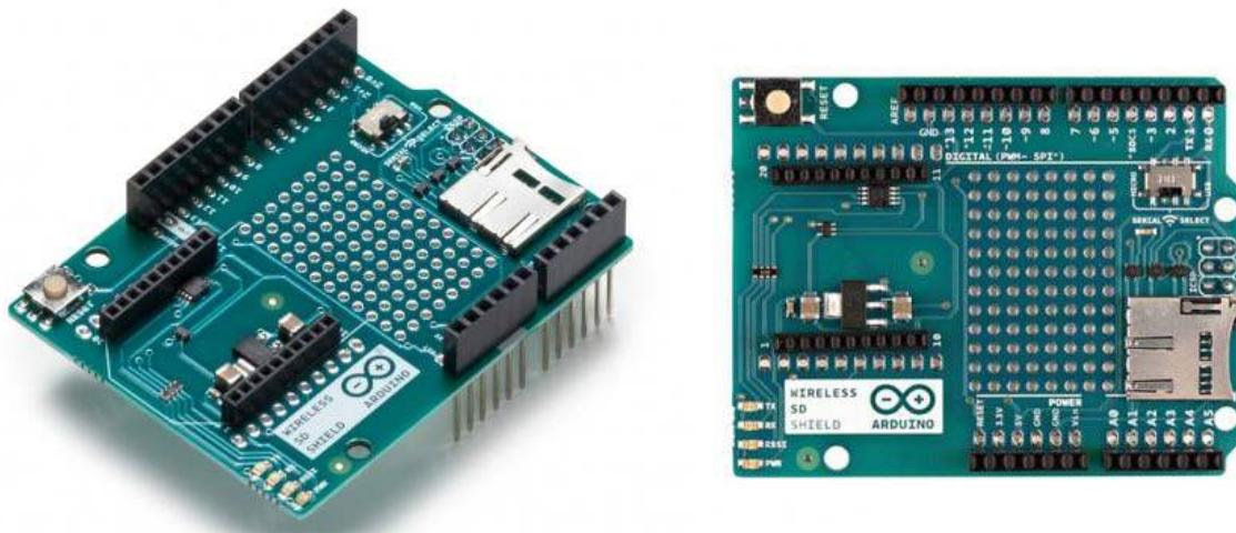
The Wireless SD shield allows an Arduino board to communicate wirelessly using a wireless Xbee module or similar plus a micro-SD card slot
