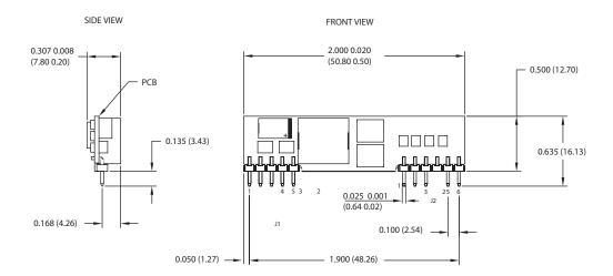
Dimensions in Inches (mm) Tolerances (unless othe rwise specified) 2 Place 0.15 3 Place 0.006
