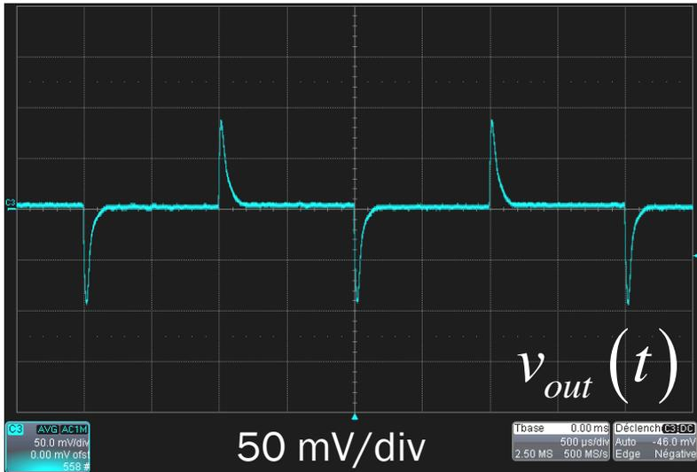
$$V_{in} = 36 \text{ V} - 2 \text{ to } 6 \text{ A} - 1 \text{ A}/\mu\text{s}$$
