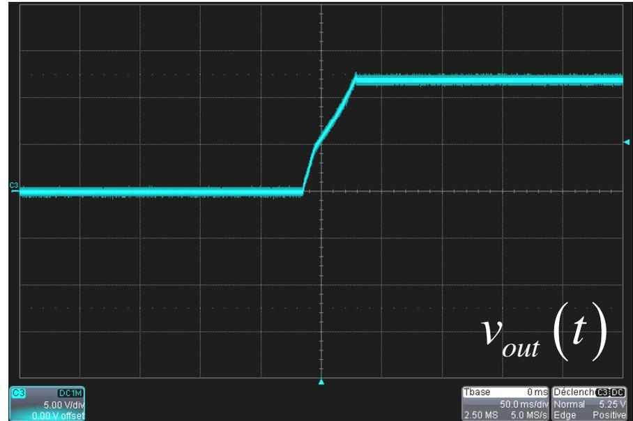
$$V_{in} = 0 \text{ to } 48 \text{ V} - I_{out} = 0 \text{ A}$$
