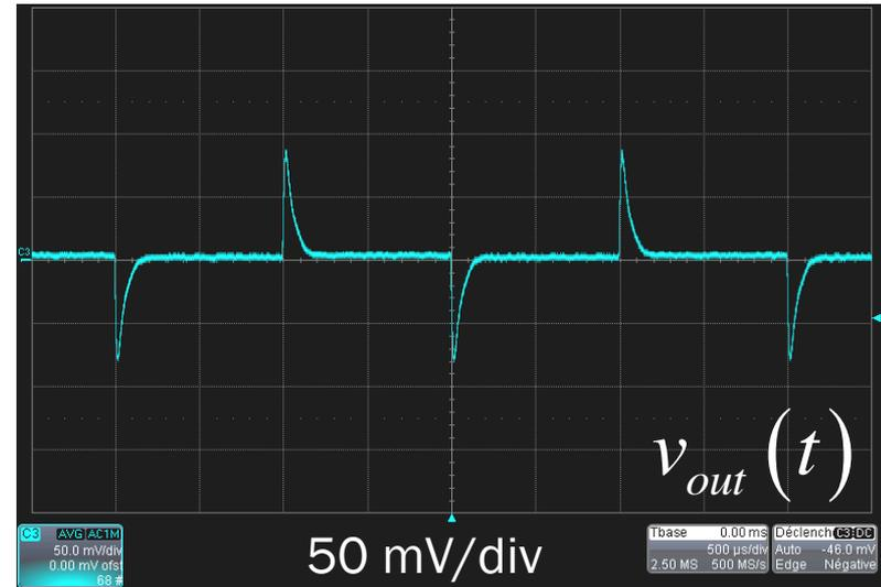
$$V_{in} = 48 \text{ V} - 2 \text{ to } 6 \text{ A} - 1 \text{ A}/\mu\text{s}$$
