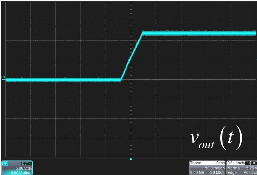
$$V_{in} = 0 \text{ to } 48 \text{ V} - I_{out} = 6 \text{ A}$$
