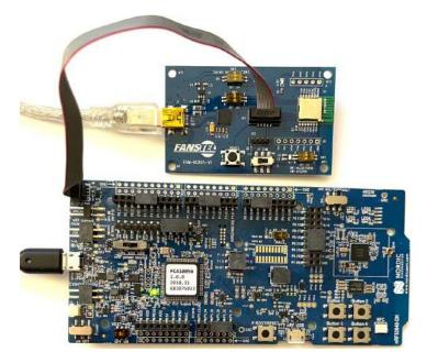
• Use *nRF Connect* to program BC805M module on the EV board.
