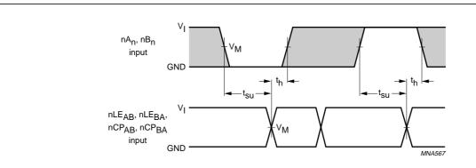
The shaded areas indicate when the input is permitted to change for predictable output performance.
