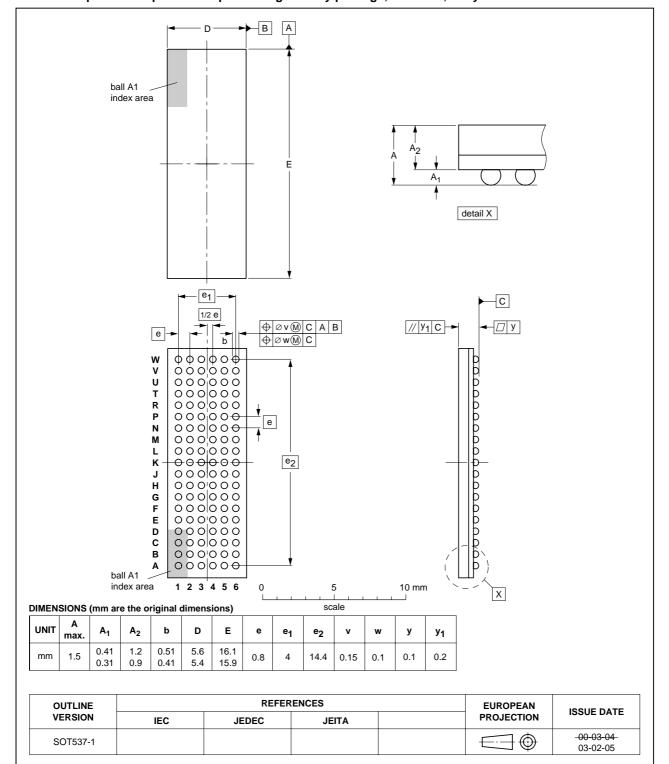
LFBGA114: plastic low profile fine-pitch ball grid array package; 114 balls; body 16 x 5.5 x 1.05 mm SOT537-1
