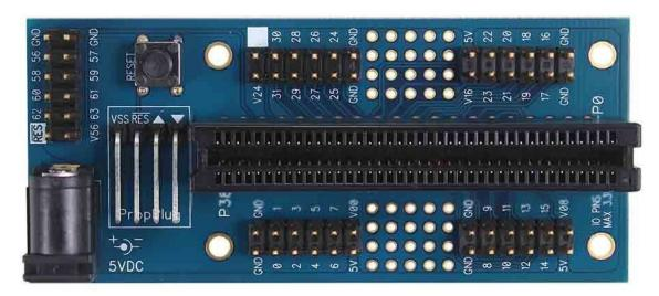
The P2 Edge Mini Breakout Board provides a compact interface to the P2 Edge Module for experimenting and developing with the Propeller 2 microcontroller.
