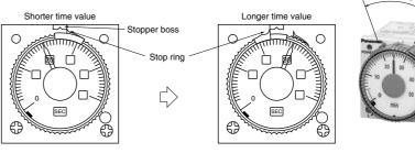
Note) The stoppers for the lower limit setting set ring and the upper limit setting set ring face the opposite directions.
