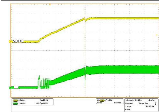
Figure 8-8. Start-up Waveforms in V_{IN} = 12\text{ V} , V_{OUT} = 5\text{ V} , R_{LOAD} = 1.2\ \Omega , FPWM
