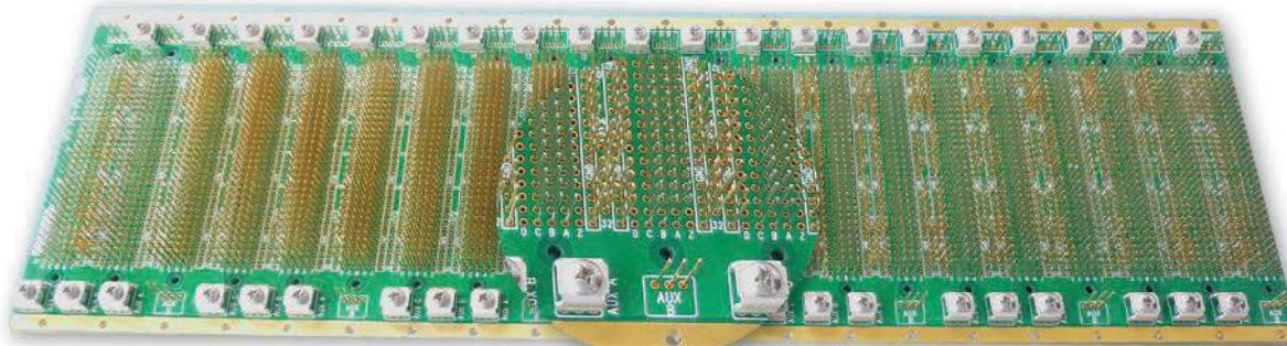
Rear View Universal (uncommitted) 3U backplane with 96 & 160 pin DIN Connector
