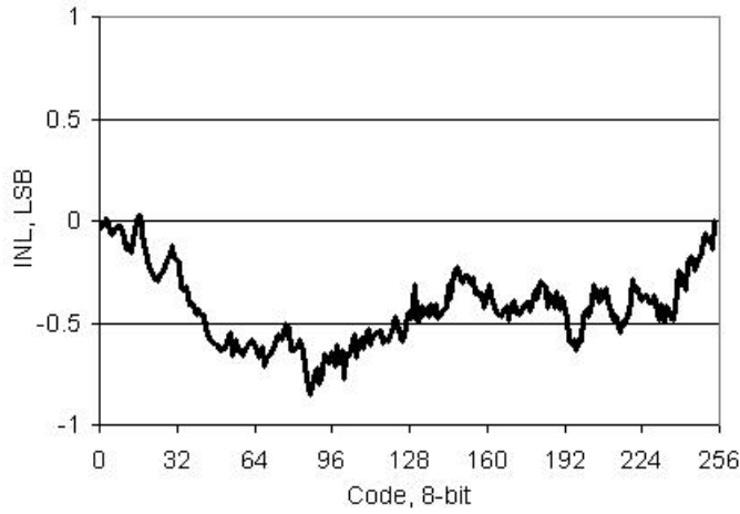
Figure 11-23. IDAC INL vs Input Code, Range = 255 \mu A, Source Mode
