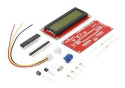
**Description:** This new revision includes a JST cable and also fixes the TX/RX swap from the last revision. Now you can use an FTDI correctly. We are also including a 16-pin header instead of a 40-pin header (only 16 pins are necessary).
