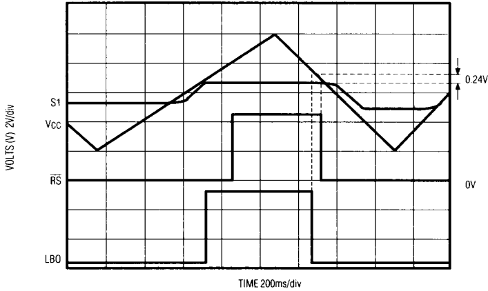
BACKUP-BATTERY SWITCHING AND WARNING FLAGS
