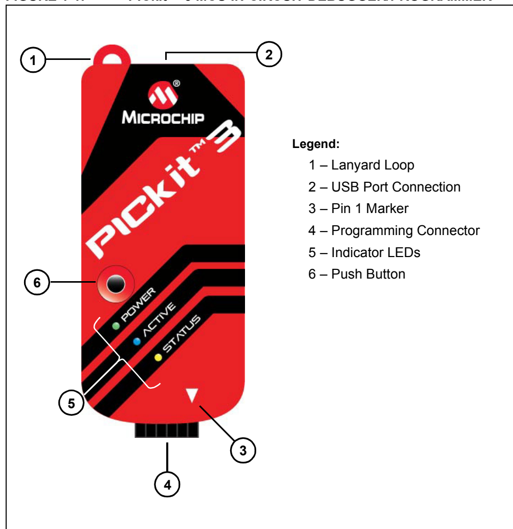
FIGURE 1-1: PICKit™ 3 MCU IN-CIRCUIT DEBUGGER/PROGRAMMER
