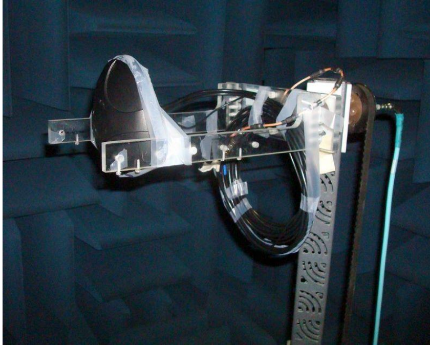
MA.600 tested in CTIA approved 3D chamber
