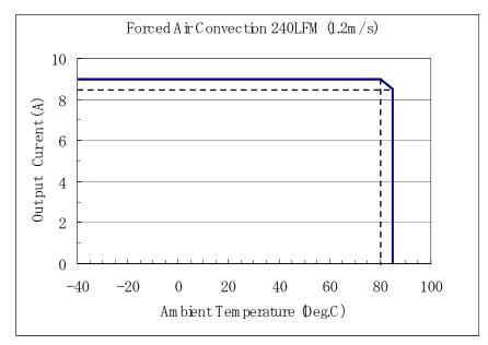
Notice:We would like to emphasize that these data are based on our experimental measurement. Please confirm that the maximum temperature of components mounted on a PCB substrate of the DC-DC Converter is 120°C or less in your application.
