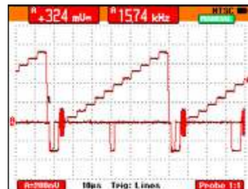
Smart averaging shows the averaged curve of repeated signal parts, as well as incidental deviations
