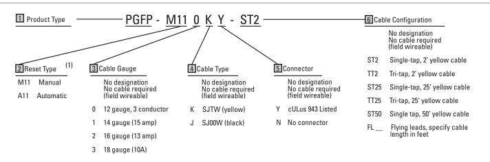
Note: 1. Manual configuration should be specified if automatic power-up, after power restoration of circuit power, could create an unsafe condition. 2. Integrated or replacement cable must be indoor/outdoor 3-conductor cable of type ST, SJT, SE, SJE, SO or SJO 3. Custom cord sets are available. Please consult Airpax for other options
