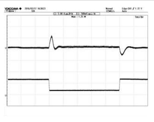
Figure 4: Dynamic response to load step 25%~75% with 0.1A/uS slew rate at 110/220Vac TOP: V_{out} , 500mV/div, BOTTOM: I_{out} , 5A/div, 1ms/div
