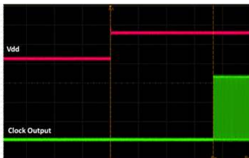
Figure 17. Startup Waveform vs. Vdd
