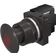
30mm BlackMax, Epoxy Coated Corrosion Resistant Complete Metal Unit Illuminated Push-Pull Operator Transformer type, 480V AC Incandescent Lamp Mushroom Head Cap Small 1 3/4" (44.5 mm) Metal, Black with Red Lens 2 Position Maintained, Pull-to-Release UL Listed, CSA Certified NEMA 1,3,3R,4,4X,12,13 & Automotive Standards
