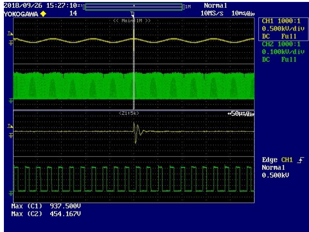
Figure 142 – (+) 2.5 kV Ring Wave Surge, 270° Phase Angle. Lower: V_{DRAIN} , 100 V / div., 10 ms / div. Peak V_{DRAIN} : 454.17 V.
