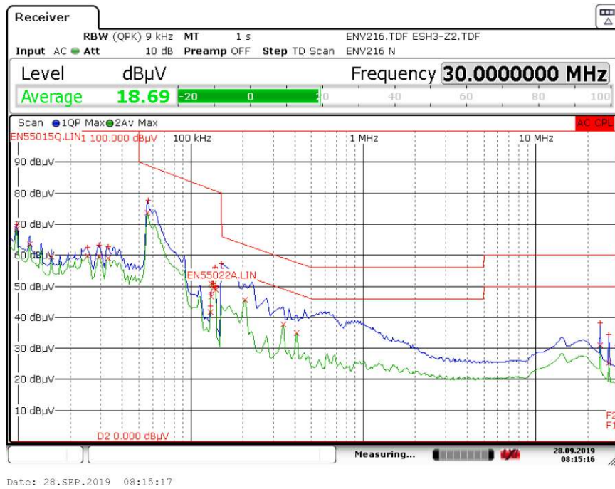
Figure 122 – Conducted EMI QP Scan at 48 V LED Load, 120 VAC, 60 Hz, and EN55015 B Limits.
