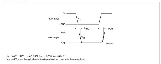
Fig.5 Input (nAn) to output (nYn) propagation delays.
