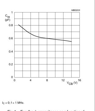
Fig.4 Feedback capacitance as a function of collector-base voltage; typical values.
