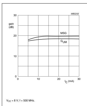
Fig.6 Gain as a function of collector current; typical values.
