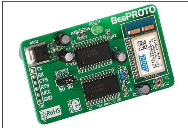
Figure 1: BeePROTO additional board
