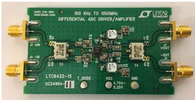
Figure 5. DC2496A Topside with Balun Installed
