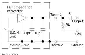
RL =  $2.2 \text{ k}\Omega$ C =  $1 \mu\text{F}$
