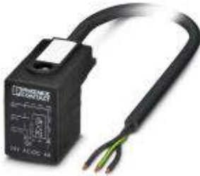
Sensor/Actuator cable, 3-position, PVC, Black RAL 9005, Free cable end, on B valve plug (10 mm), with 1 LED, connected with Z diode, Cable length: 10 m
