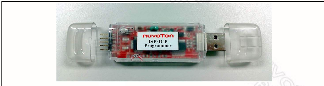
Figure 27-2 Nuvoton ISP-ICP Programmer
