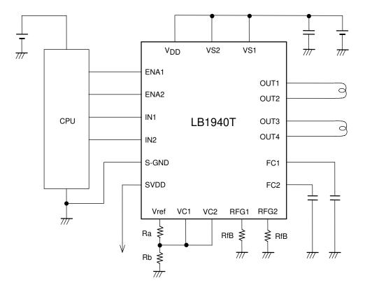
At constant-current control: The OUT current is controlled so that the RFG pin voltage is equal to the VC input pin voltage.
