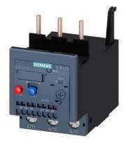
Overload relay 9...12.5 A Thermal For motor protection Size S2 Class 10 Contactor mounting Main circuit: screw terminal Auxiliary circuit: spring-type terminal Manual-Automatic-Reset
