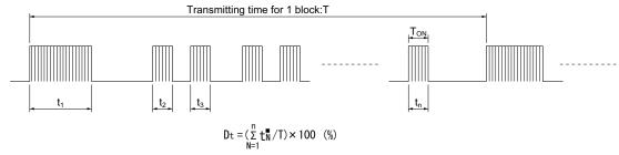
In case the signal format of total duty and/or ON/OFF signal time dosen`t meet the conditions noted above, there is a case that reception distance much reduces or output dose not appear.
