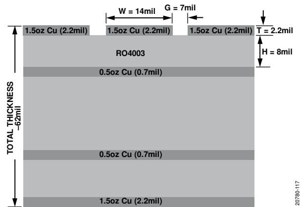
Figure 17. Probe Matrix Board Stack Up
