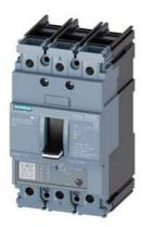
circuit breaker 3VA5 UL frame 125 3-pole, starter protection TM120M, AM, In=80A without overload protection short-circuit protection li=5...12 x In cable connection on both sides
