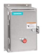
Non-reversing motor starter Size 1 Three phase full voltage Solid-state overload relay OLRelay amp range 0.25-1A 220-240/440-480VAC 60HZ coil Combination type Water/dust tight non-corrosive
