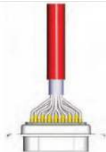
Strip cable 18mm and shape cable to two pigtails
