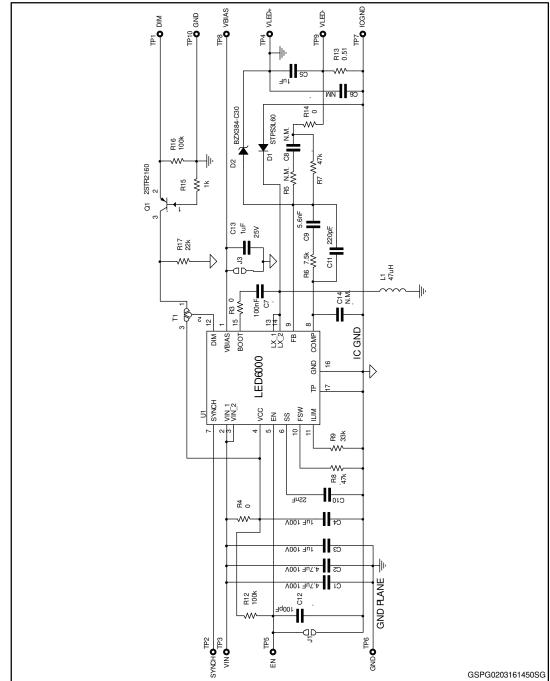
Figure 1: STEVAL-ILL079V1 circuit schematic
