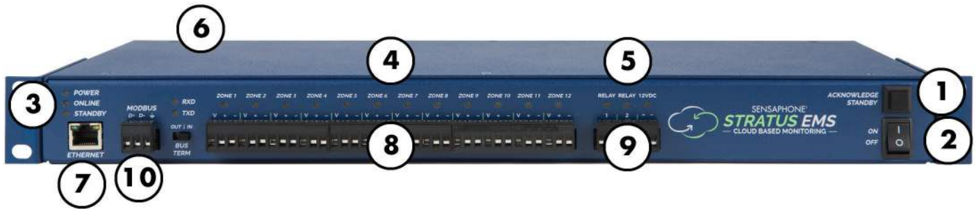
Figure 1: Front Panel Layout of the Stratus EMS
