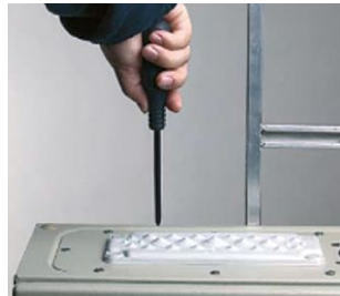
Make a small hole in the membrane.
